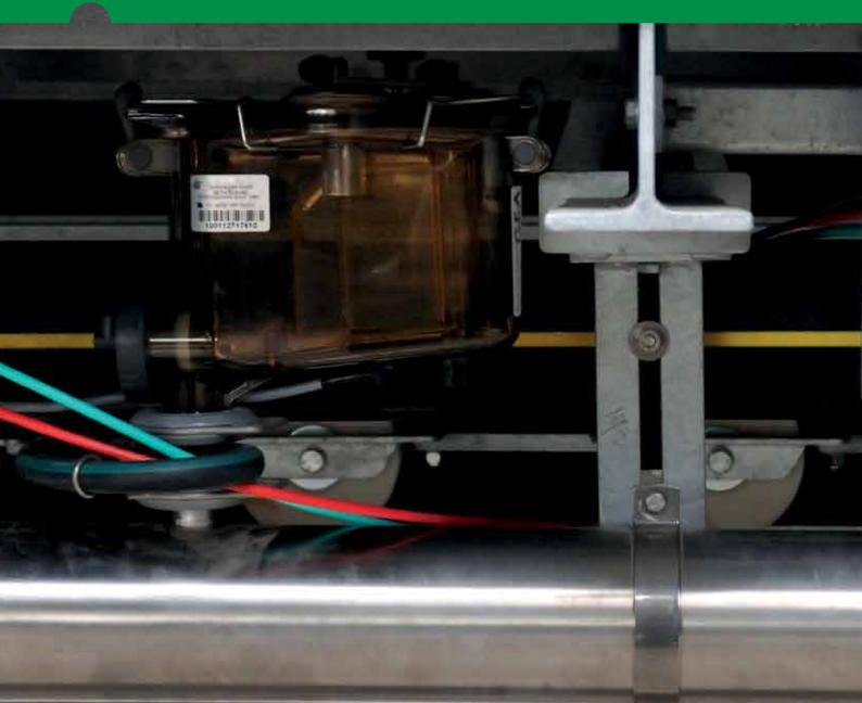
This way the feeding tub is locked into place in the interjacent stall along with the tub from the entrance, so there's ample space for the cow to leave the platform. As soon as another cow enters, a plastic leaf spring pushes the feeding tub back into its position, upon which the runner secures the tub. Since the stalls have been made 20 centimetres longer, there's extra space and time to get off the platform.
